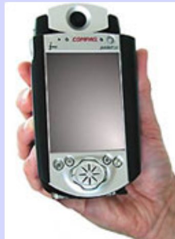
Compaq's iPAQ with MIT Oxygen Project camera sleeve
